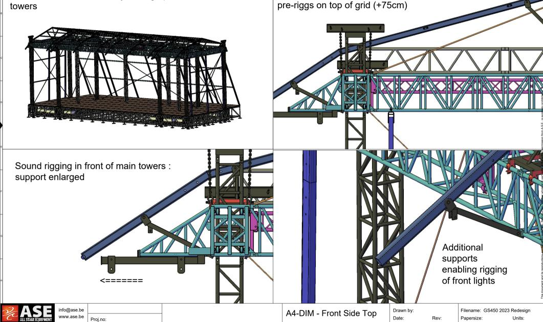
Increased clearance through increased height of roof structure support => possibility to place up to H52
