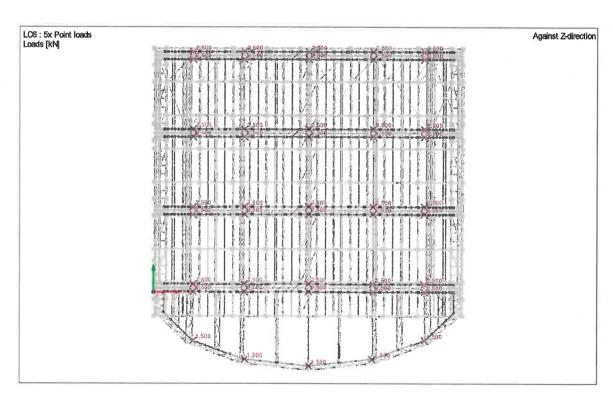
The loading which is taken into account in the 5x Point loads setup are: Arche Truss = 5x 500 kg Cantilever Truss = 5x 150 kg
