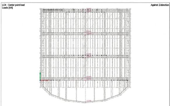
The loading which is taken into account in the Centre point Load setup are: Arche Truss =  $1x\ 1000\ kg$  Cantilever Truss =  $1x\ 350\ kg$
