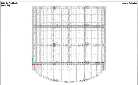
The loading which is taken into account in the 2x Point loads setup are: Arche Truss = 2x 700 kg Cantilever Truss = 2x 350 kg
